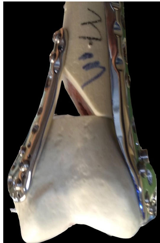
Fig. 1 AP view of a Group 2 sample (DFLP+PHLP). Note the orthogonal arrangement of the plates. The model was mounted upside down on the testing machine, with an adduction angle of 10 degrees to reproduce physiological load transmission, and the load was applied to the condyle through a polymeric component of a knee prosthesis
