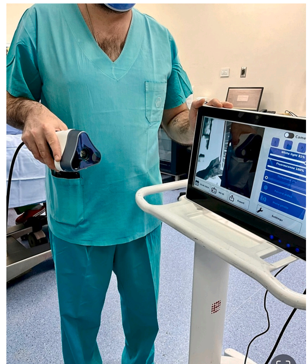
Fig. 1. Dendrite® Imaging system. The Dendrite® Imaging system employs a near-ultraviolet light (NUVL) source and filter system to detect fluorescent signals emitted by neural tissue. These signals then pass through a filter system within the camera head, are captured by a chip, and are transmitted to a dedicated software platform for real-time analysis, processing, and relay to a display screen, allowing the surgical team to observe neural structures clearly fluorescing.
